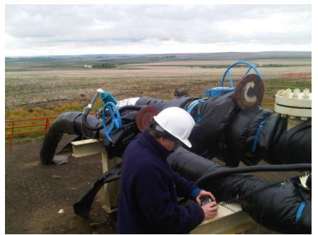
Figure 1.2.1 - Simulated Leak Point and Gas Flow Measurement Equipment.
