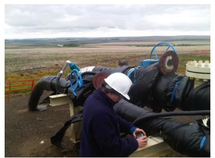
Fig. 1.3.2 – En Cana Staff Measuring Gas Leak Flow Rate
